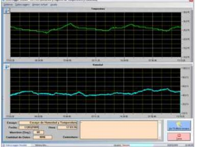
The Data Logger Reader - DS1923 is a software that allows reading and Configuring DS1923 Loggers. These data loggers record temperature and humidity every time. The user must set the interval (between 1 seg. to 273Hs min.).
